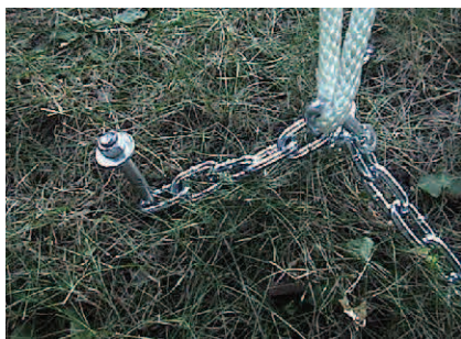
With the stakes pounded in at a slight angle, the chains pull sideways and won't slip up the stakes.
