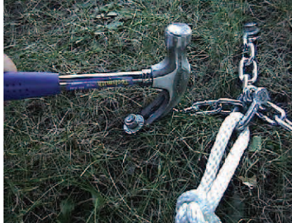
A small hammer in the tiedown kit bag will be handy to both pound in the stakes and get them back out.
