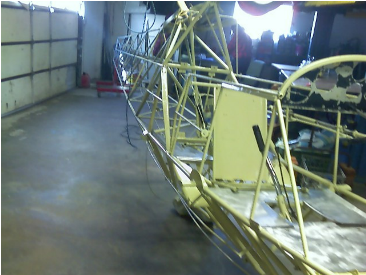
N2689 Fuselage in shop for recovering.
